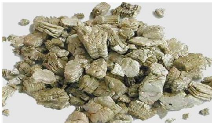
Picture 7 – Expanded vermiculite of the Kulantau deposit (Turkestan region)
