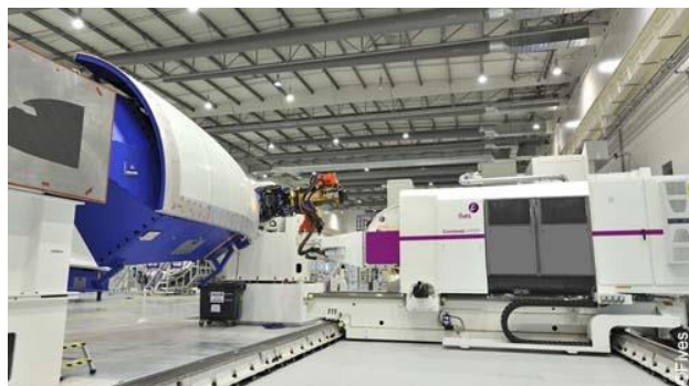
Fig. 4 Machine for automated winding-laying out of Viper 1200 FPS angle fillers by MAG Cincinnati
